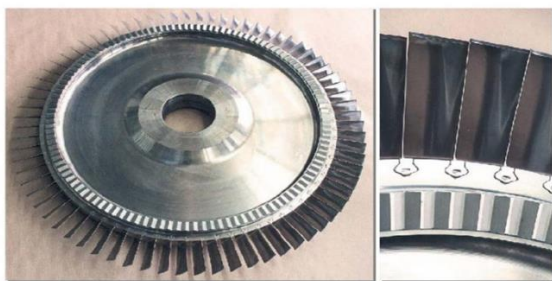
Figure 4. Gas turbine compressor disk V94.2
