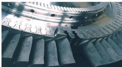
Figure 9. V94.2 turbine moving blade disc
