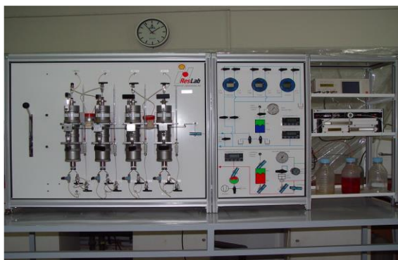
Figure 2. Formation resistivity factor apparatus under overburden pressure, Research Institute of Petroleum Industry
