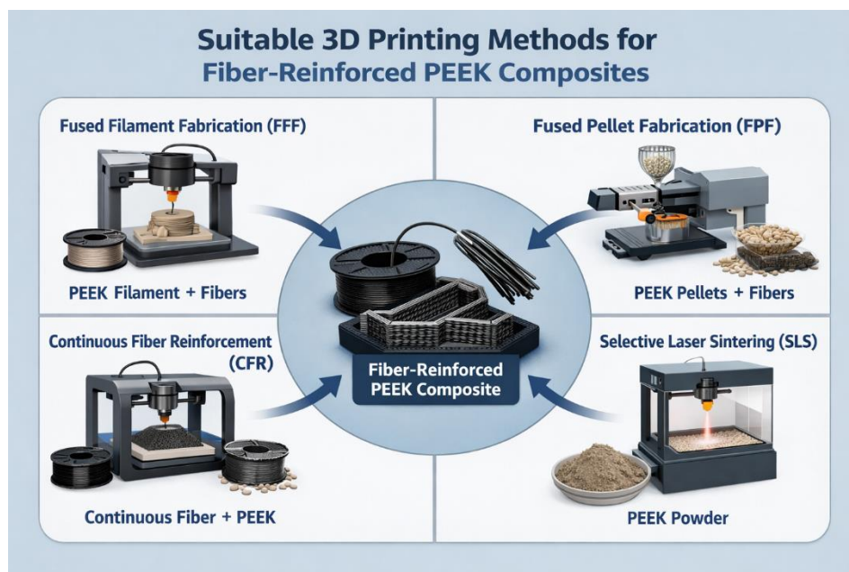
Figure 5. Suitable 3D Printing Methods for Fiber-Reinforced PEEK Composites
